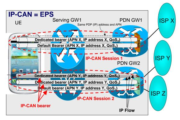
Figure 1: IP-CAN, IP-CAN Session, IP-CAN Bearer and IP Flow
