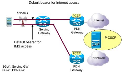
Figure 3 : Connectivity for Internet Access and IMS access when the user is in his home
