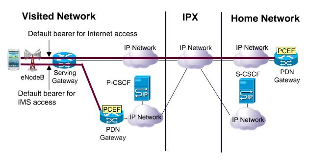
Figure 6 : Connectivity for Internet Access and IMS access when the user is in a roaming situation
